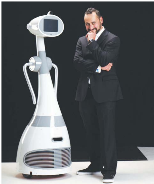
FIGURE 3: RoboDynamics' new Luna (shown here with company CEO Fred Nikgohar) is a 5 ft., 2 in. open-standard hardware platform featuring feature a native App Store, standard PC architecture, an open Linux-based operating system, touchscreen display, Wi-Fi and multiple USB ports for expandability.
